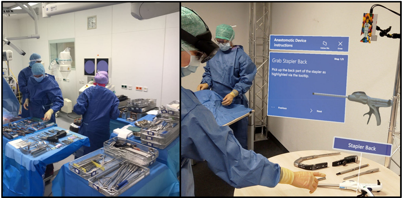
Fig. 1 Example of the amount of surgical instruments being used during surgery (left) and photomontage concept of assembly guidance with HMD on the users head and static camera analyzing the surgical tray (right)
